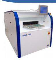
The VAC 745/765 (available as batch or inline) combines the advantages of the vapor phase with the vacuum process and guarantees void-free solder joints with highest quality. The soldering system operates in a completely inert atmosphere during the whole reflow and vacuum process. Many patented features are available and provide a wide range of flexibility. The machine promises oxygen-free soldering an no overheating of components. In addition, the power consumption of the machine is very low.
