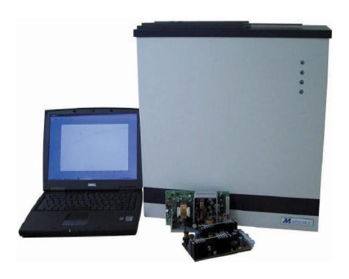
The CT10 is designed to make simple and accurate ionic contamination test on big boards (up to 100x150 mm) in fully compliance with MIL-P-28809, MIL-STD-2000A, DEF-STD 10/03, IPC-TR-583, IEC Standards...
