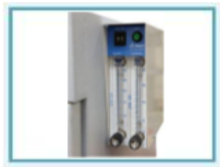
N 2 Autoflow system The autoflow system is developed to use in combination with a Totech drying cabinet. The device is used for the quick removal of moisture in the cabinet after the doors have been opened. The drying process is realised by using Nitrogen (N 2 ), which is purged automatically after the doors are closed. (timer controlled) Item number 22613001
