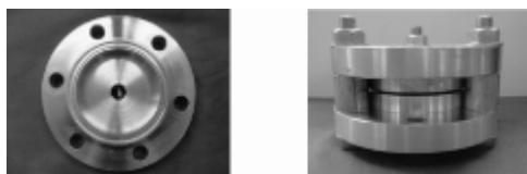
Figure 6. Flange for pressure resistance test
