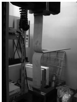
Photo-2. Appearance of T-type peeling test
