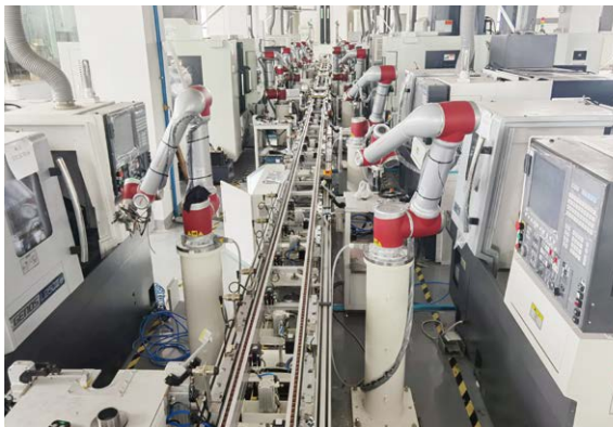
Loading and Unloading
