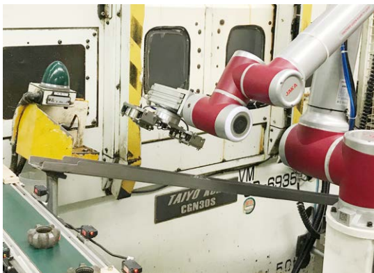
Loading and Unloading
